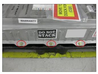
4. Securely fasten the HV Battery metal cover to the base of the battery with **ALL original** fasteners.
