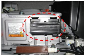
1. Cover the hybrid battery service plug terminal with UL-listed non-conductive black electrical tape.
