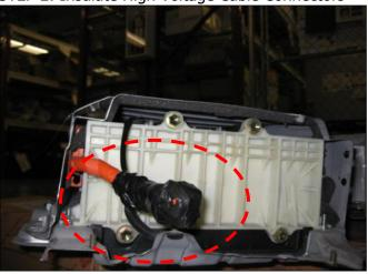
2. Cover all exposed high voltage cables, wire harnesses and or terminals with UL-listed non-conductive black electrical tape.
