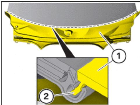
① Push the cowl top ventilator louver sub-assembly into the claw ② beginning on the side
