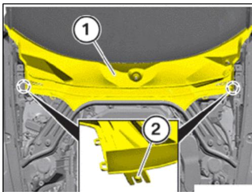
① Engage the cowl top ventilator louver sub-assembly in the claws ②
