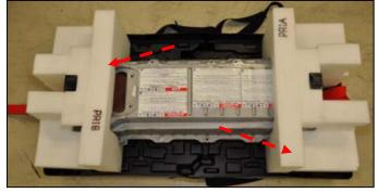
3. Install the foam end caps onto the battery.
