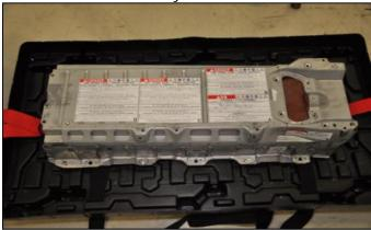
1. Place the battery in the center of the DRC.
